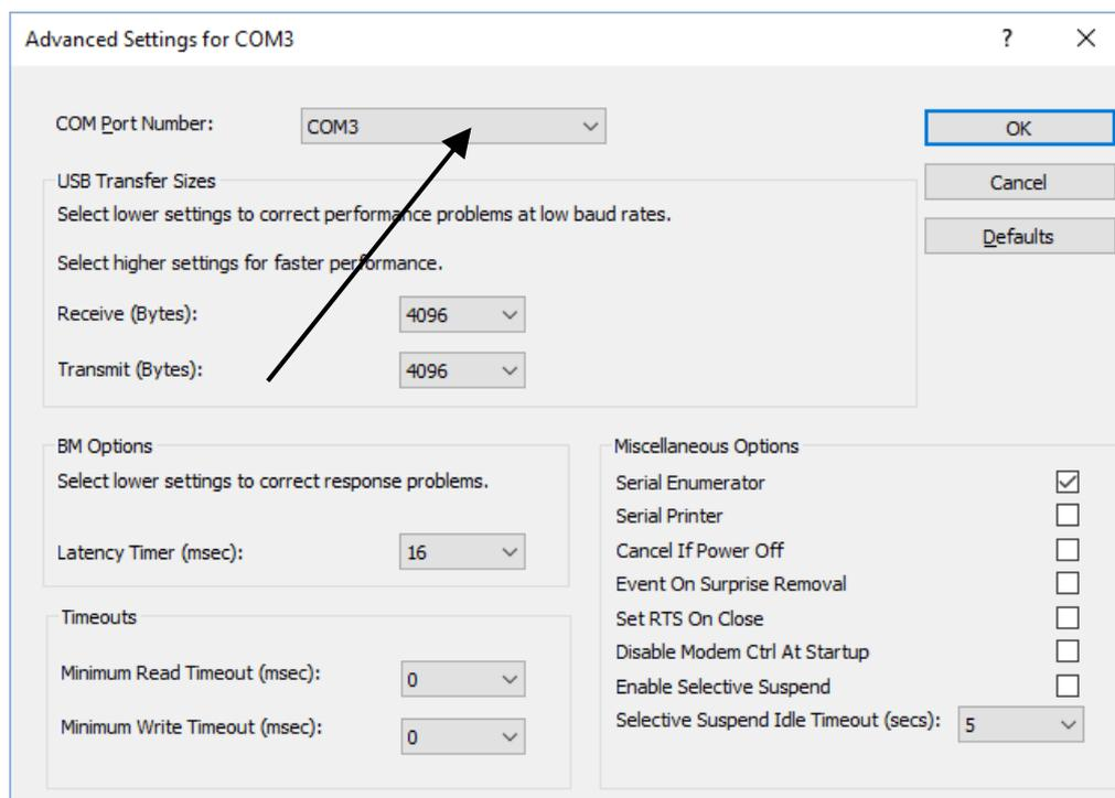
Select a free port number between COM3 and COM8. Remember this number for the adjustment of the Interface-Program.
