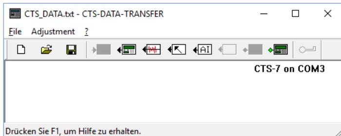
With "Adjustment" you select the COM-Port number you have pinned after the installation of the FTDI driver. In this example COM 3.
