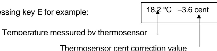
By pressing key "E", you enter the actual instrument program. The actual cent setting in the instrument program is not influenced by the cent adjustment of the thermosensor. For the creation of the target frequency, both values (thermosensor- and actual cent adjustment) are added up. In the tuning program, the sensor is reanalyzed. The evaluation also occurs during the recording of a tone at least once per minute
